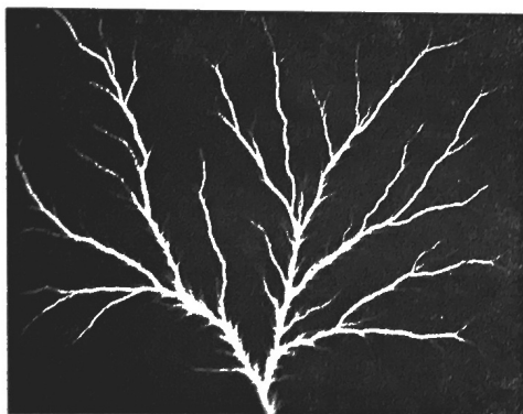
Fig. 1 A few minutes after receiving 0.2 megarads 6 Mev electron dose this block was lightly tapped with a sharp point producing this self-illuminated photograph.
