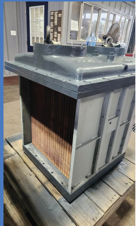
Here's a Marine Application After Cooler from the team at Don Hart Radiator in Texas that was cleaned, tested, and repaired before being shipped out.
