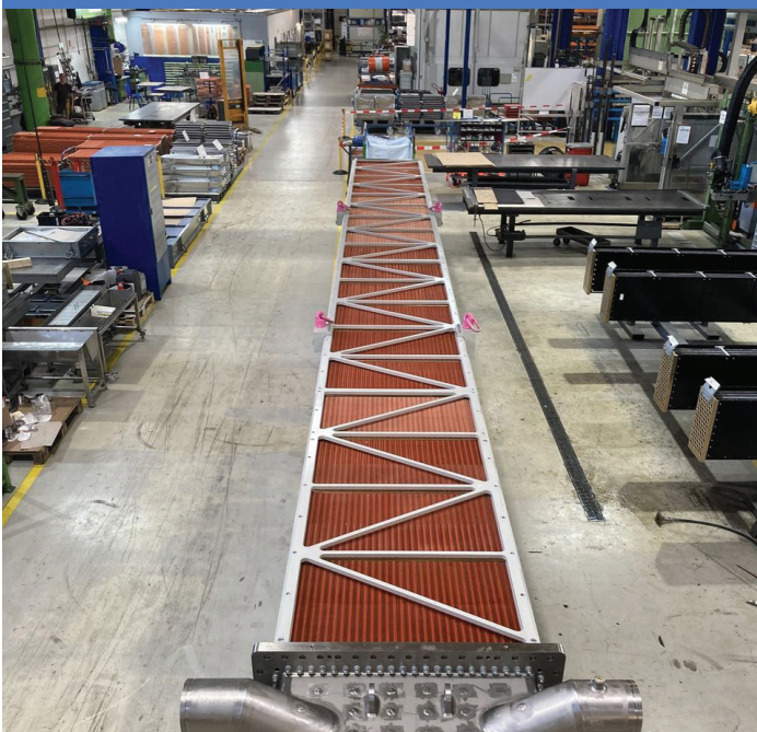
The latest work from Kelvion's team in Herne, Germany. They have manufactured an impressive Closed Circuit Cooler for the energy industry. Crafted from a combination of titanium and copper, this cooler boasts a net weight of 11,500 kilograms and stretches over 12 meters in length.
