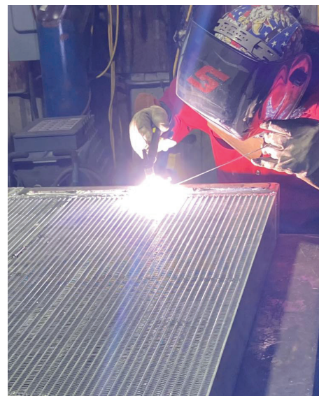
Check out this Recore of a 3 pass Lube Cooler from the team at Industrial Radiator Service in Dallas, Texas.
